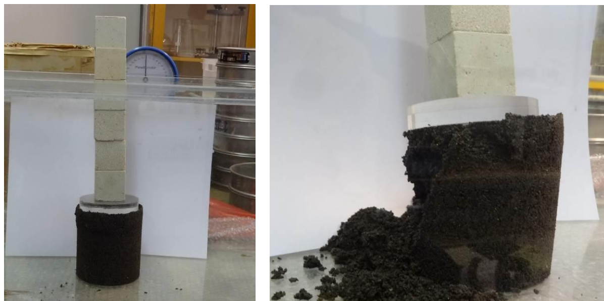
Figure 22. High bearing capacity of wet unsaturated sand.
