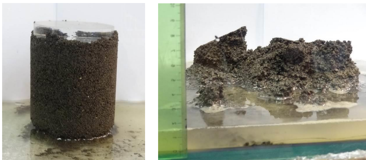
Figure 23. Initial phase of failure of sample loaded by water.
