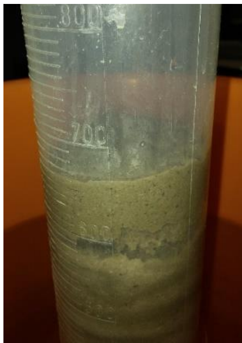
Figure 19. Upheaval of saturated sand layer by pore air pressure increase in partly saturated sand.
